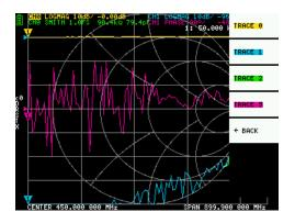
Up to four traces can be displayed, one of which is the active trace.
