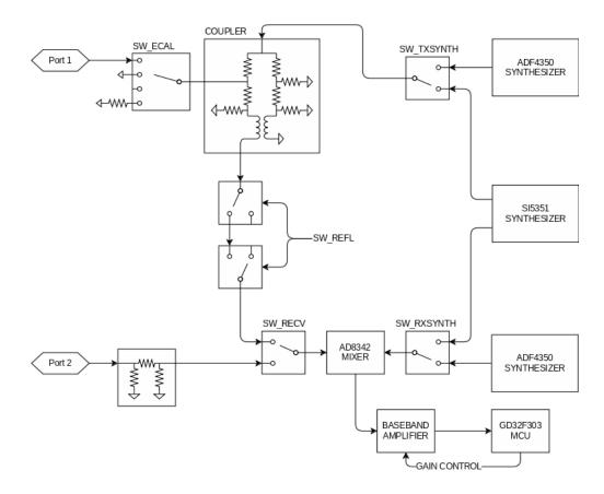
The NanoVNA V2 is a single switched receiver VNA. While the diagram shows only two channels selectable by the receive mixer through SW\_RECV, a third channel, the reference channel, is provided by setting SW\_ECAL to the "open circuit" position. By controlling these two switches the receiver is able to observe reference, reflected, and thru signals.
