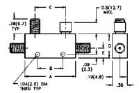
Midwest Microwave's SMA miniature series of Ultra-Wideband high performance directional couplers are small, lightweight, components that perform extremely well over multi-octave and Ultra-Wideband frequencys covering the entire range of 0.5 - 18.0 GHz.
