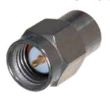
Midwest Microwave's series of Plug and Jack Mismatches are conveniently offered in all of the popular connector interfaces. They are particularly useful for performing phase measurement tests. The units are available in eight standard mismatch values and special versions are available on request. All of the units are finished in passivated stainless.
