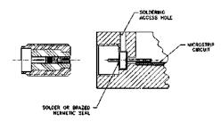
Drop-in Assembly - Feedthru Connector
