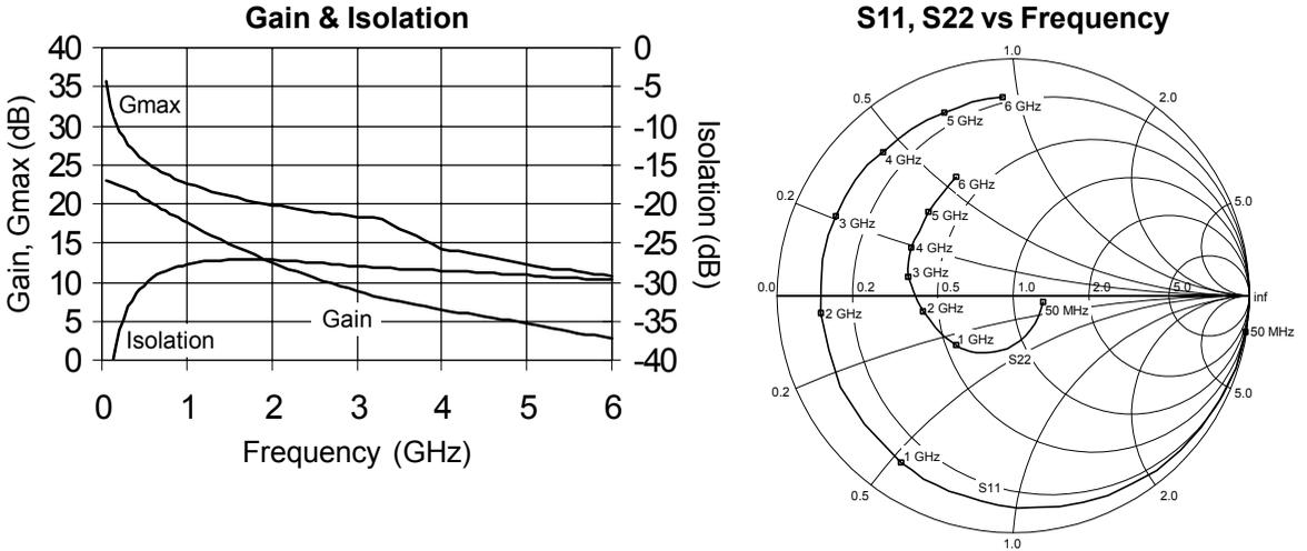
Note: S-parameters are de-embedded to the device leads with  $Z_s=Z_L=50\ \Omega$ . The data represents typical performance of the device. De-embedded s-parameters can be downloaded from our website ([www.sirenza.com](http://www.sirenza.com)).
